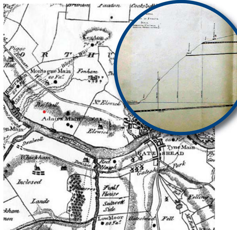
Extract from 1801 map showing coalmines in Newcastle with (inset) cross-section of strata at Benwell showing the High Main coal seam outcropping at or near St James'.
